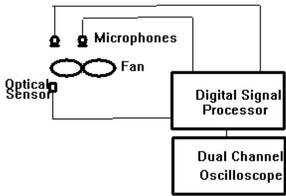
Figure 1. Sound Field Testing System.
